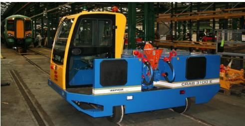
Fig-11:- Battery Tractor
